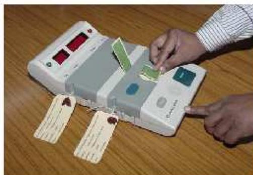
**Step 2:** Keep the Strip Seal with the pre-gummed portion .A. positioned near the base of the inner fold of the Green Paper Seal protruding from the inner side of the outer door of the Result Section. Remove the wax paper over .A. and press the inner fold of the Green Paper Seal over this gummed portion and paste.
