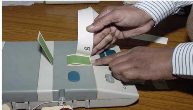
**Step 4:** After pasting 'B' over the Green Paper Seal the pre-gummed portion 'C' will come to the top position. Remove the wax paper over 'C', press the Green Paper Seal protruding from the top portion of outer door so that the Green Paper Seal is firmly pasted over 'C'.
