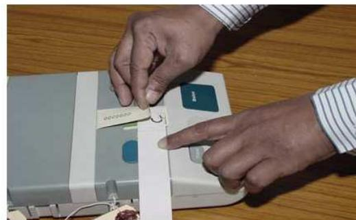
**Step 5:** Take the remaining portion of the Strip Seal round the Control Unit from left side taking care that the strip passes below the 'CLOSE' Button. Bring the other end of the Strip Seal from right side of the Control Unit on top of the outer door where the pre-gummed portions 'A', 'B' and 'C' have been pasted.
