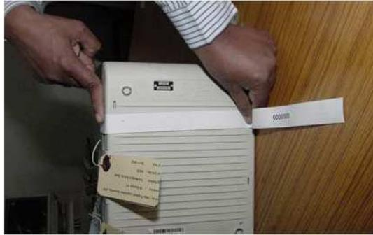
**Step 6 :** Remove the wax paper covering the pre-gummed portion 'D' and press it firmly over the Green Paper Seal protruding from the top portion of the door. The pre-gummed portion 'D' spills over the Strip Seal below the 'CLOSE' Button. Press this spilled over portion of 'D' firmly over the Strip Seal.
