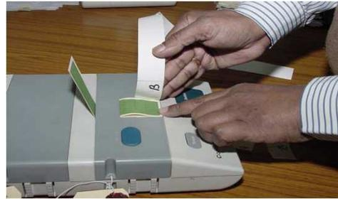
**Step 3:** Remove the wax paper over the pre-gummed portion .B. and press this gummed portion over the outer fold of the Green Paper Seal.
